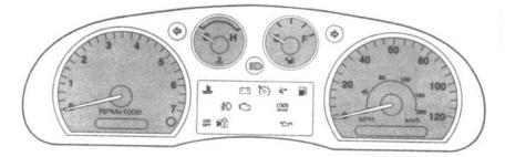
Speedometer: Indicates the current vehicle speed.
