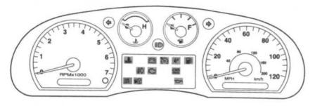
Warning lights and gauges can alert you to a vehicle condition that may become serious enough to cause expensive repairs. A warning light may illuminate when a problem exists with one of your vehicle's functions. Many lights will illuminate when you start your vehicle to make sure the bulb works. If any light remains on after starting the vehicle, refer to the respective system warning light for additional information.
