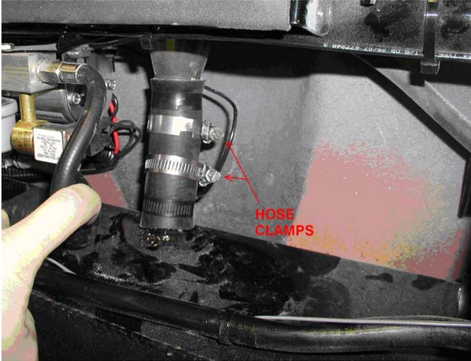
7. Remove Air Compressor and Junction Block from Frame
