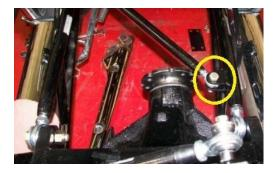
If jam nuts on panhard bar (pictured below) have been locked down, back off jam nuts & turn adjusting bar until side to side adjustment is even between left and right tires (DO NOT TIGHTEN JAM NUTS YET). The panhard bar can be accessed by reaching up between the rear end and the trunk.
