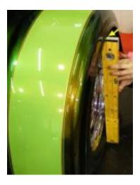
If side to side is not the same and needs to be adjusted, loosen the jam nuts on the diagonal bar and disconnect diagonal bar from right rear ladder bar connection point (see below).
