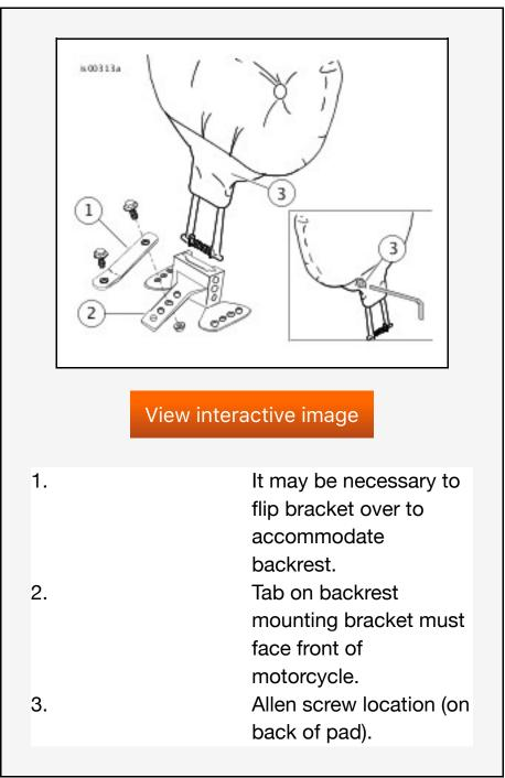
Figure 1. Backrest Support and Bracket Position
