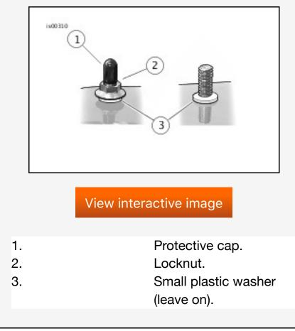
Figure 2. Leave Bottom Washer Attached (1999 Models)
